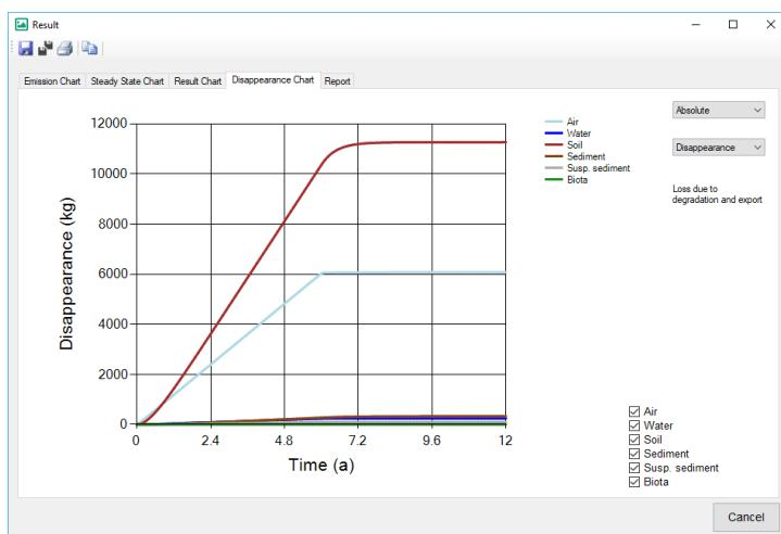
**Figure 10: Disappearance chart: Change of degradation in the environmental compartments in time**
