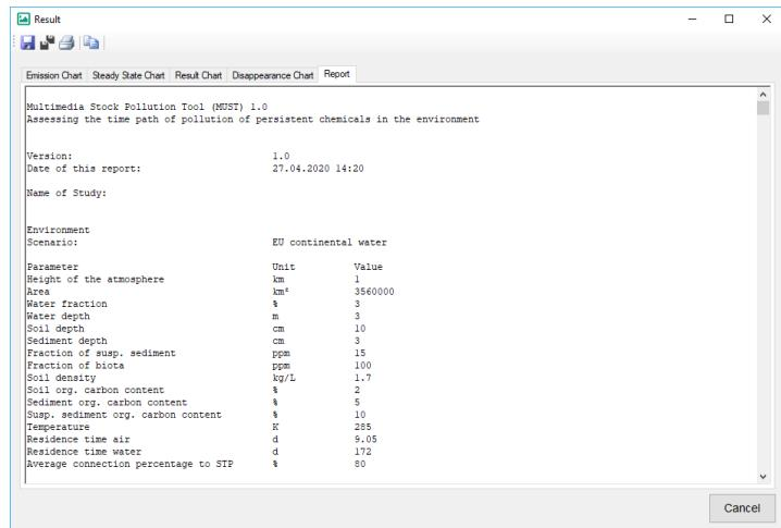
**Figure 11: Text report file containing the input data as well as the calculation result**
