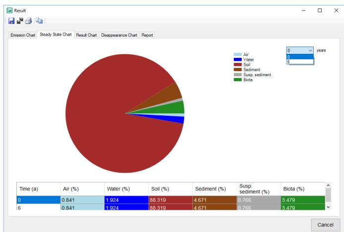
**Figure 8: Steady state chart. Result of Mackay III calculation, distribution of mass in the environment in long term perspective**
