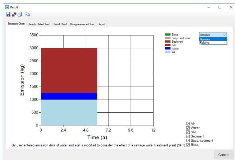
**Figure 7: Input chart: emission data after sewage water treatment plant (SPT)**
