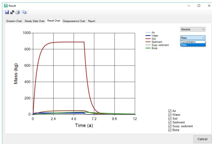
**Figure 9: Result chart: Change of mass in the environmental compartments in time**
